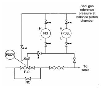
Figure 6: Differential Pressure Control - Courtesy of American Petroleum Institute -
