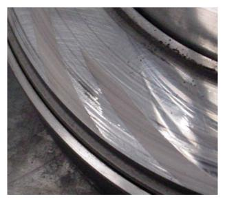
Figure 8: Scratches on the Mating Ring
