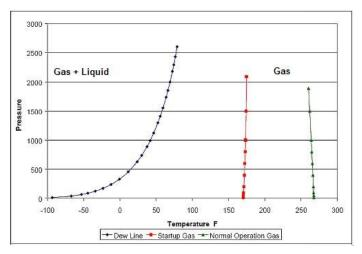
Figure 9: Seal Gas Phase Diagram
