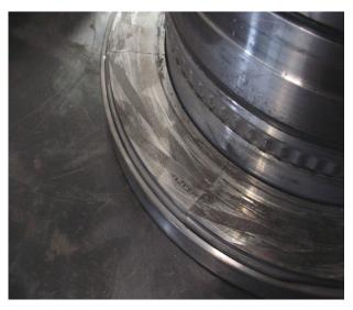
**Figure 7: Damaged Mating Ring**
