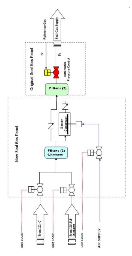
Figure 10: Seal gas conditioning system
