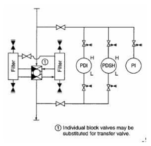
Figure 5: Seal Gas Filter Module - Courtesy of American Petroleum Institute -
