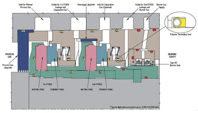
Figure 3: Cross-sectional view of a Typical Tandem Gas Seal
