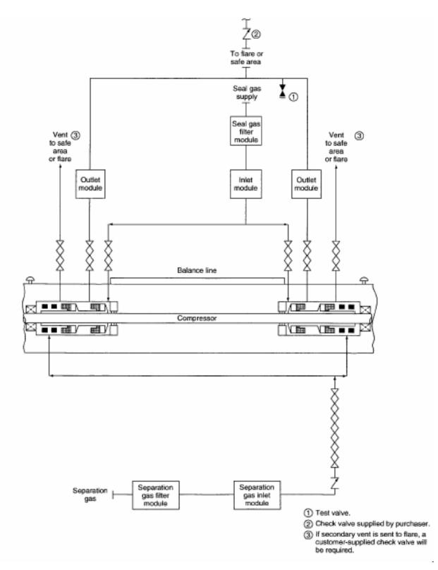
Figure 4: Tandem Dry Gas Seals Support System Schematic - Courtesy of American Petroleum Institute -
