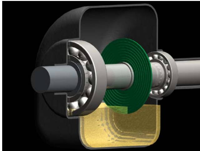
Fig. 4: Shaft-mounted flexible flinger disc splashes lube oil into bearings (Ref. 2) (Source: also
