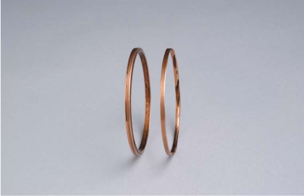
Fig. 6: Oil rings in as-new (“wide and chamfered”) condition on left, and abraded (“worn and narrow”) condition on right side (Source: Ref. 2)
